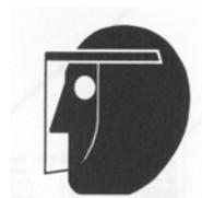
Face shields are recommended when you see this symbol. Face shields protect against splashing and crop debris, but are not designed for high-impact hazards (projectiles). Use industrial safety glasses under the face shield for complete protection.
